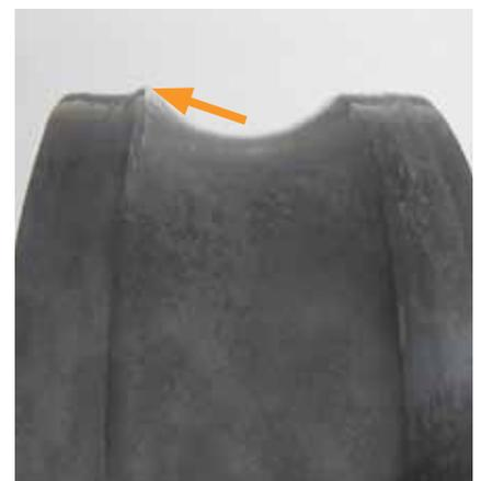
Softening and deformation of the thrust shoulder caused by excessive loads. The discoloration on the inner ring is the result of elevated temperatures.
