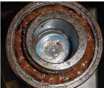
Lubrication characteristics of the grease are compromised by water ingress.
