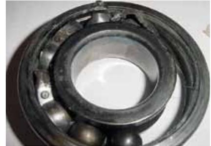
Metal cage damage due to misalignment or excessive speed.
