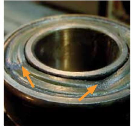
Seal damage due to improper installation procedure and/or tools.
