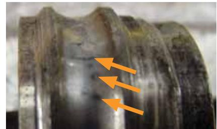
Wear caused by vibration or axial movement between the balls and races in a static condition.
