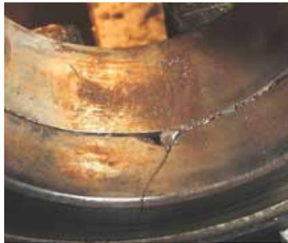
Inner ring cracking due to excessive taper on the shaft.
