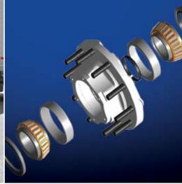
The type of wheel bearing system you use can have many service implications. There are three main types of wheel bearing systems you will find in the field. These systems are: adjustable, pre-adjusted and unitized. By identifying the type of system you have, you can then determine the type of service to be performed.
