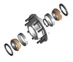
the nut acts to retain it on the spindle. This type of wheel-end system cannot be serviced in the field. The entire system will need to be replaced. You cannot replace separate components.
