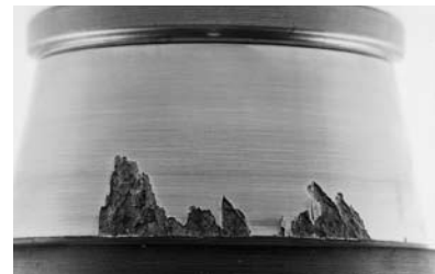
Fig. 2 – Geometric Stress Concentration (GSC) spalling
