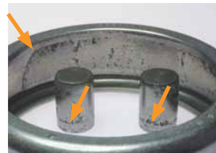
Cylindrical bearing outer race and rollers with peeling and moderate wear due to underfilling of lubricant.
