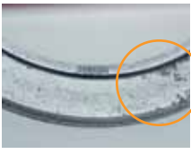
Fig. 3 - Needle thrust bearing inner race peeling (micro-spalling) due to thin lubricant film from elevated temperatures.
