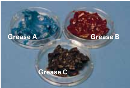
Fig. 5 - Grease A and Grease B are not compatible. When mixed together they become lumpy, discolored and hard in composition (Grease C).
