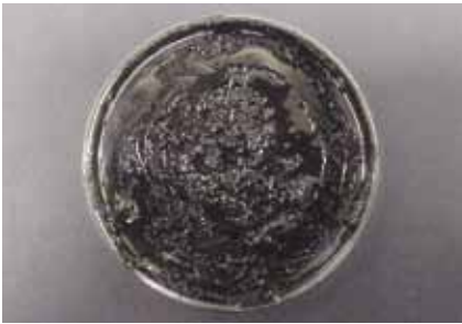
Fig. 2- A petri dish containing heavily oxidized grease, which purged from an overfilled bearing. Grease undergoing heavy oxidation often has a very
