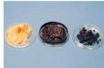
Fig. 8 - The above photo shows the same grease at three stages (from left to right): 1) new grease, 2) heavily oxidized grease, and 3) worn-out (failed) grease – the thickener and additives have decomposed and the oil is breaking down.
