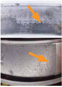
Fig. 4 - Peeling: Micro-spalling in a tapered roller bearing outer race (above) and inner race (below) due to thin lubricant film from elevated temperature.
