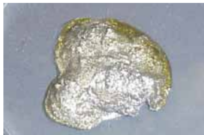
Grease removed from an underfilled bearing showing shiny bearing metal debris.
