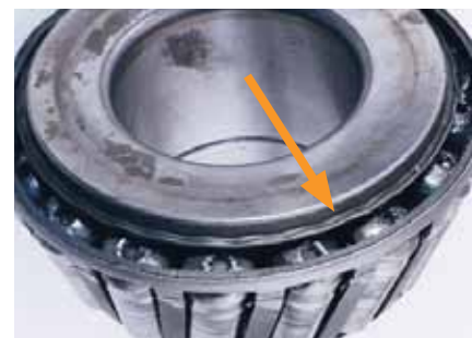
Tapered roller bearing cone large rib face deformation: Metal flow from excessive heat generation.
