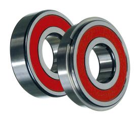
When standard clutch pilot bearings are operated in these higher temperature environments, the seals start to breakdown and the grease liquefies. This allows the grease to be purged past the bearing's seals and a loss of lubricant inside of the bearing. Bearings operating without any lubricant quickly become noisy and ultimately fail.
