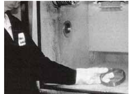
Thermostatically-controlled freezer units aid in the installation of tight-fitted cups in hubs.
