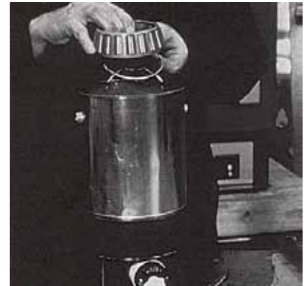
Hot oil pots, with a tray or hook to support the cone, effectively ease the installation of tight cones on shafts.
