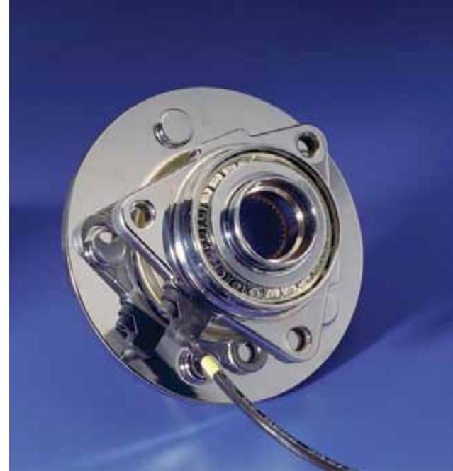
external sensors can be damaged from excessive movement caused by too much end-play. This indicates a lack or loss of bearing clamp. This normally results from severe mechanical break up or damage. (Additionally, in designs where the sensor is mounted externally, sensor damage can result from corrosion, stones and other hazards.)
