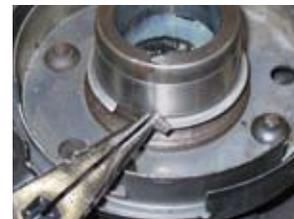
**9)** After the Kwik-Sleeve is installed, check again for nicks or burrs that could damage the seal.
