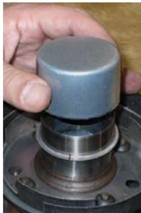
**7)** Gently strike the center of the installation tool with a large, soft-faced mallet until the sleeve covers the worn seal surface. If thread repair compound was used, thoroughly clean off any
