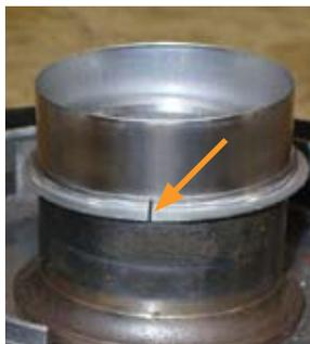
**5)** Fill deeply scored grooves with a thread repair compound. Place the sleeve onto the shaft before the compound hardens. The
