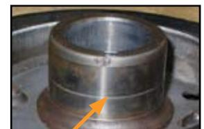
*If you can catch your fingernail in a shaft groove or seal wear track, a Kwik-Sleeve can be installed to prevent leakage.*
