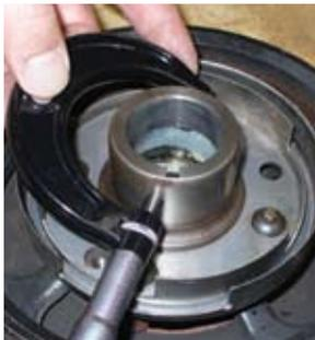
**3)** Determine the sleeve position necessary to cover the old seal wear grooves. Measure to the exact point, or mark di-
